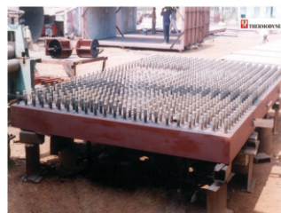
FLUIDISED BED COMBUSTOR
